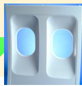
Honeycomb panels (around windows)
