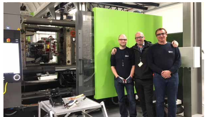
Weighing 500 tons, one of the world’s largest machines for thermoset injection molding (sbDRIVE Demo Center)
