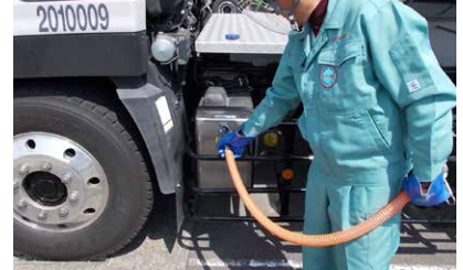
Sunbake We installed an automated supply system for Adblue (for detoxifying nitrogen oxide) at a distribution hub in Shizuoka City.
