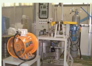
Supercritical testing equipment
