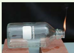
Recovered gas ignition test
