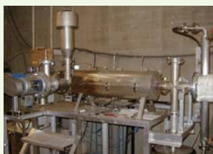
Horizontal moving-bed type gasification experimental unit
