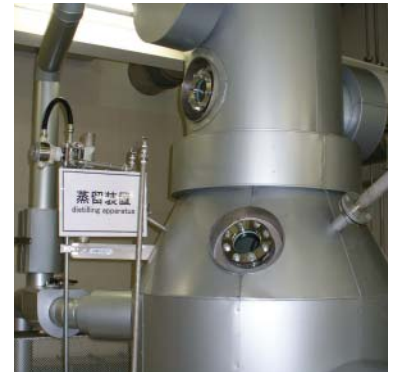
Distillation recovery equipment for waste isopropyl alcohol
