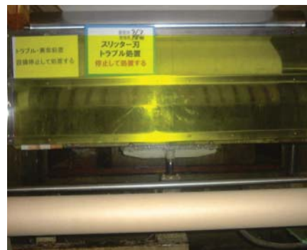
Shield to prevent items from getting caught in impregnating equipment (Artlite Kogyo Co., Ltd.)
