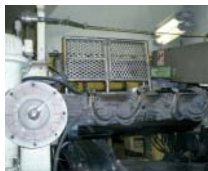
Safety fence installed to prevent potential danger from contact with a roller (Utsunomiya Plant)
