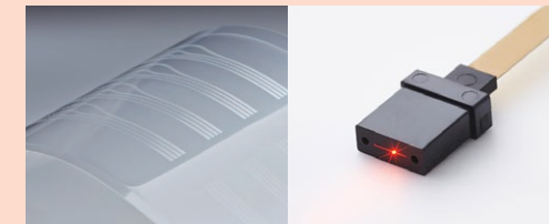
Optical circuit film (left photo) and Polymer waveguide with optical connector (right photo)
