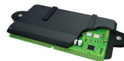
Direct encapsulation materials for ECU
